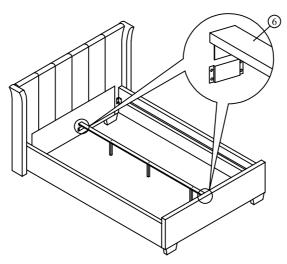
Step 6: Insert the bottom panel (14) to the below frame and secure using hardware part J and a screwdriver (not provided).
