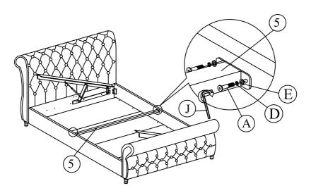
Step 9: Assembly the small wooden frame (13) and big wooden frame (14) to the bracket and tighten all the fitting accordingly.
